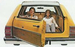
Your Chevrolet Caprice Classic or Impala Station Wagon features a three-way doorgate that swings wide to let people enter the available rear-facing third seat. Or a quick turn of the key and you can lower the glass for easy access to the rear. The door will open sideways with the glass up or down.
