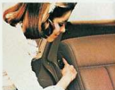
Easy seat conversion. A fingertip push on the button-type latch releases the second seat and moves it forward. Glide the seat down to its closed position and the conversion is complete.
